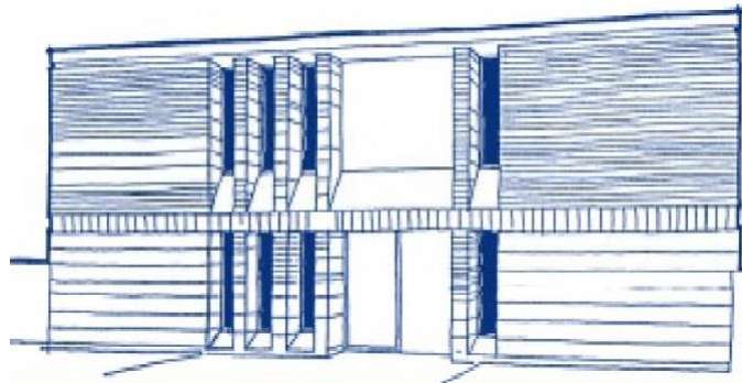
Figure 55. Narrow and recessed Windows
