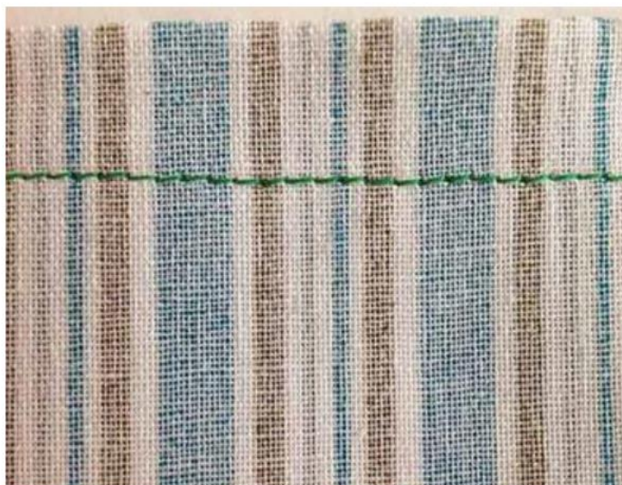
Fig. 5. Plain seam construction
