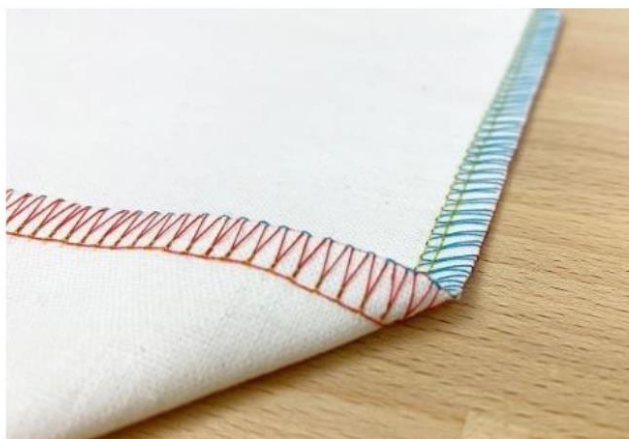
Fig. 6. Overlock (serged) seam construction
